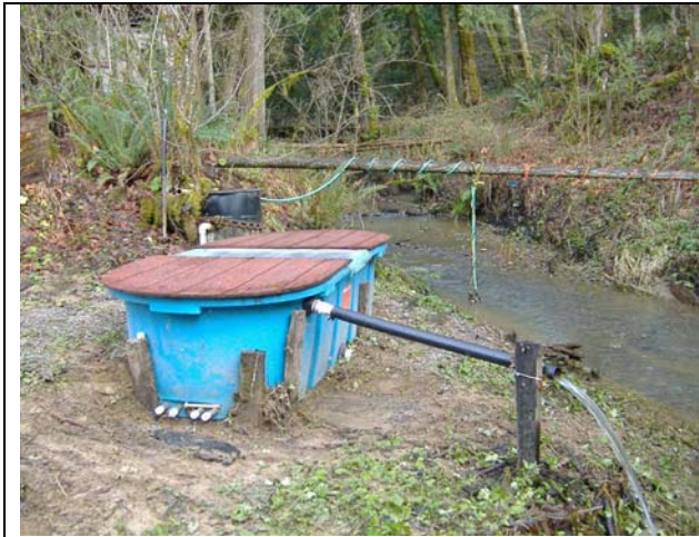
1 - Example streamside incubation system using a plastic tub.
