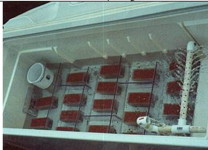
3 - Streamside incubator with Whitlock-Vibert boxes holding incubating eggs in an old freezer.
